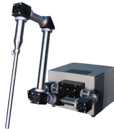
Figure 2: DMD-270 Diamond ATR Probe coupled to a Bruker IR Cube FTIR spectrometer by means of a custom Axiom interface.
