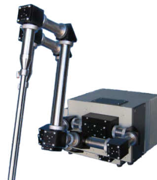
Figure 2: DMD-270 Diamond ATR Probe coupled to a Bruker IR Cube FTIR spectrometer by means of a custom Axiot interface.
