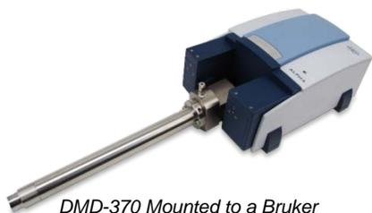
*DMD-370 Mounted to a Bruker Alpha FTIR spectrometer*
