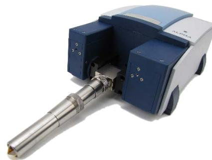
*DPR-212 Mounted in a Bruker Alpha FTIR Spectrometer*
