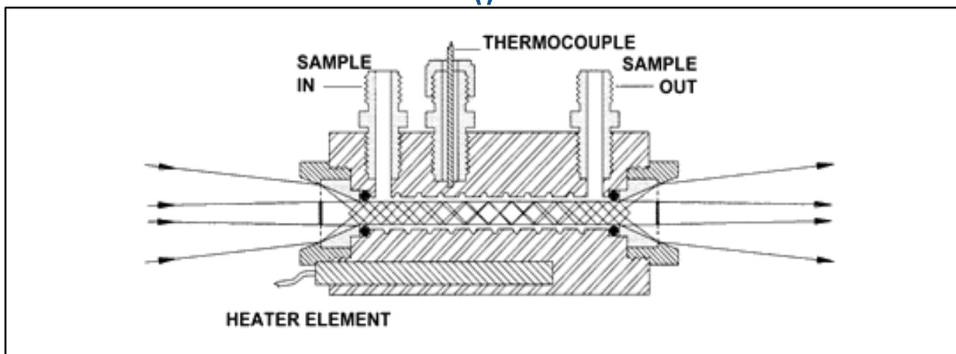
**Figure 1:** Model TNL-130H with a typical focused sample region optical geometry. The Tunnel optical design maximizes the collecting aperture while minimizing the distribution of rays within the ATR element. For the example shown (f:4 optics), the extreme rays are confined to a range of  $\pm 1.8$  degrees within the element.
