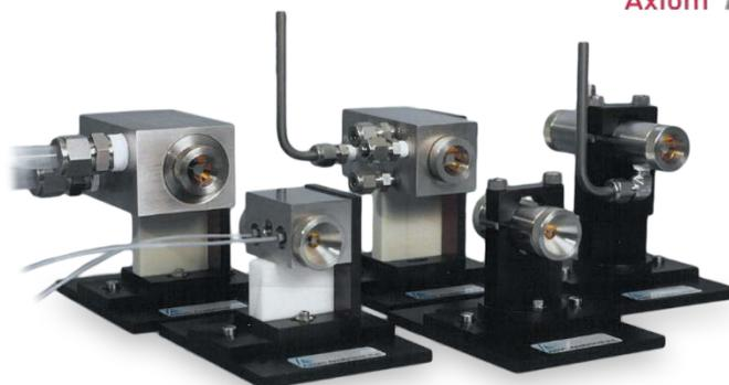
Axiom Tunnel Cells<sup>1</sup> provide both the high degree of analytical accuracy and the rugged reliability required for diverse demanding analyses. As a result, these devices can create new opportunities for FTIR Spectroscopy in application areas ranging from supercritical fluid analysis and HPLC detection, to process methods development and even the instrumentation of large process reactions.
